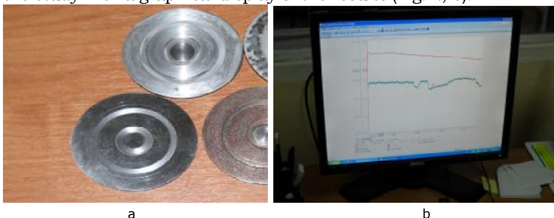
Fig. 2. Samples for tests (a) and graphical representation of the results of research on tribometer TRB – S – DE (b)
